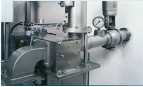
Product feed with CIP dosing system
