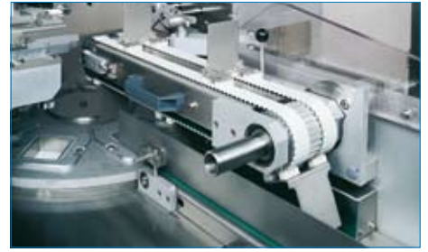
Evacuation and discharge conveyor
