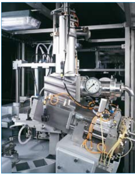
CIP cleanable dosing unit with direct product feed from the process plant
